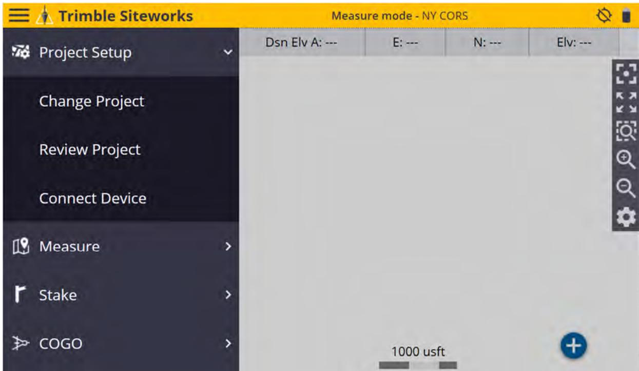
\*In **Connect Device** tap on the blue **GNSS Icon** to enter **Receiver Setup** screen.
