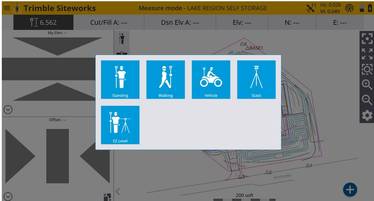
\*On the **Vehicle Mode Settings** screen if you are using a quick release select **Yes** from the **Using Quick Release** window drop-down menu. Input the Antenna height in the **Vertical height** window. (*Usually 2 Meters/6.562 usft*)
