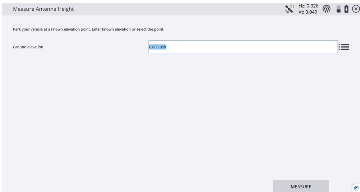
\*You can also tap the **3-Dot/3-Bar Icon** to the right of the **Ground elevation** window to access the **Select point** screen and tap on a point to reference it's elevation, tap **ACCEPT** to get back to the **Measure Antenna Height** screen.
