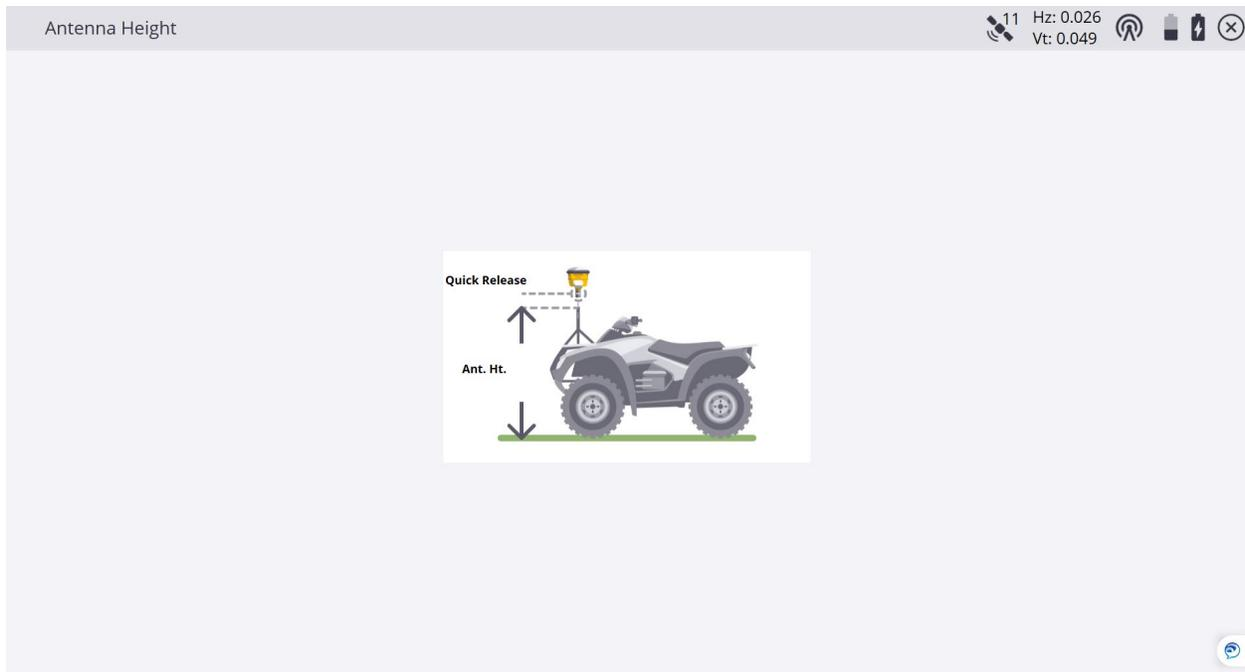
\*On the **Vehicle Mode Settings** screen to the right of the **Vertical height** window tap the **Ruler Icon** to enter the **Measure Antenna Height** screen and input an elevation in the **Ground elevation** window.
