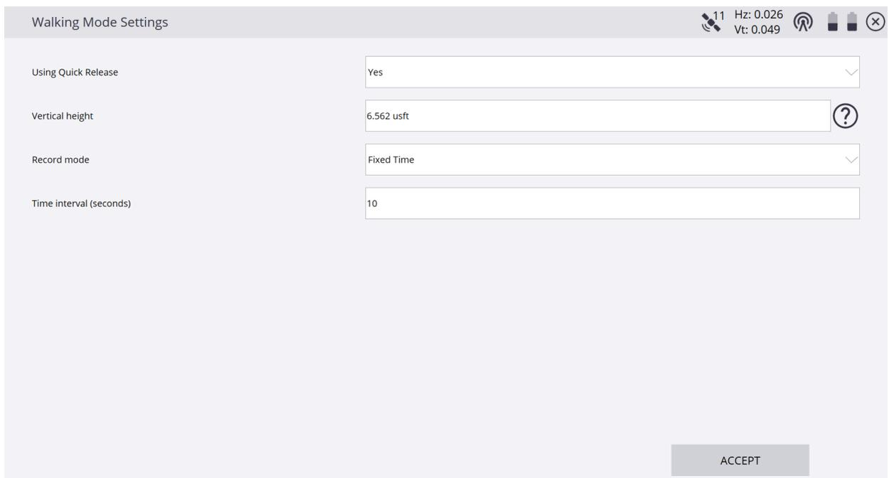
\*On the **Walking Mode Settings** screen select **Measure When Level** in the **Record mode** window drop-down menu, then input your desired values for **Tilt tolerance** and **Time interval** (in seconds) in their corresponding windows.
