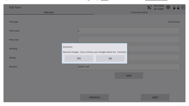
Tap <u>SAVE</u>, then tap X in the upper right corner of the <u>Edit Point</u> screen to exit the <u>Edit Point</u> screen and return to the <u>Point Manager</u> table.
