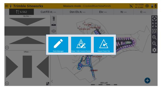
\*In the upper right corner of the <u>Point Manager</u> table tap the point <u>Count:</u> (gear cog) to access the <u>Point Manager Settings</u> screen. (There are 1720 project points)
