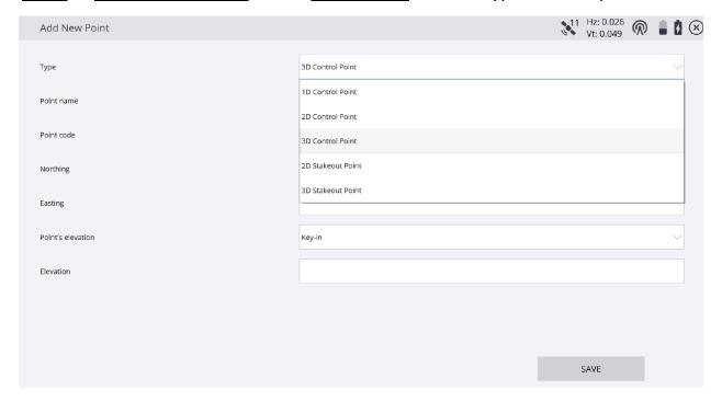
\*Tap in the <u>Point code</u> window and type the description code of the point to be created. Tap in the <u>Northing</u> and <u>Easting</u> windows input their corresponding coordinate values of the point to be created.
