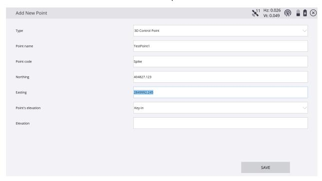
\*In the <u>Point's elevation</u> window select the elevation reference from the drop down list <u>extract from point</u> (an existing point), <u>extract from surface</u> (current working surface), or <u>Key-in</u> the elevation of the point to be created, tap <u>SAVE</u>.
